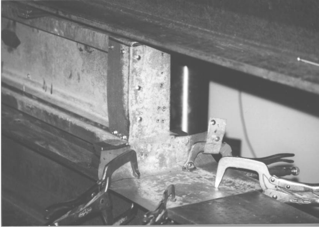
FIGURE 3 End Condition of the Header Specimens
