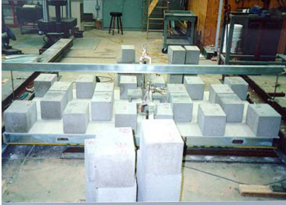
FIGURE 3 Test specimen with a 25 psf lateral load.
