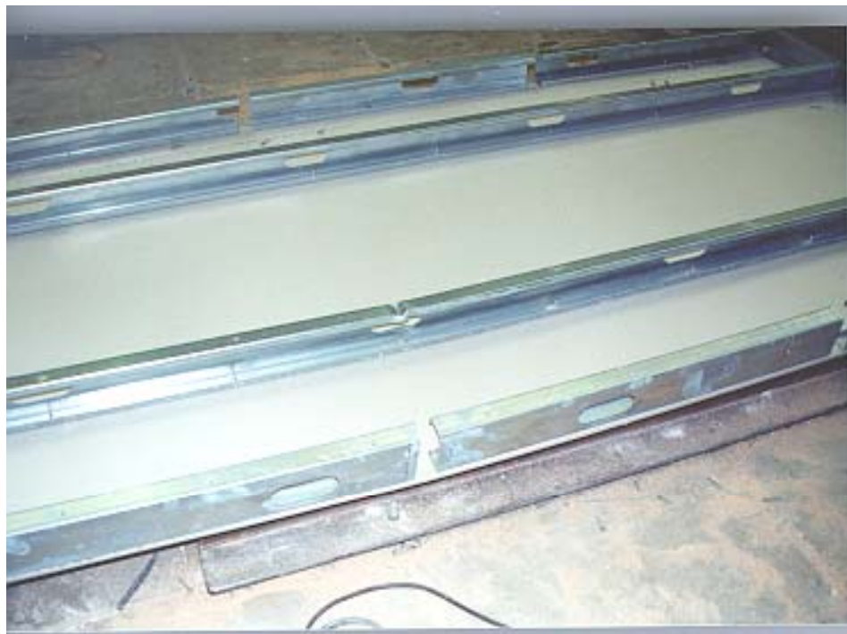
FIGURE 4 Failure of a 2x4x33 mil wall stud due to local buckling of the compression flange at a web punch-out with a 25 psf or 50 psf lateral load (sheathing has been removed).
