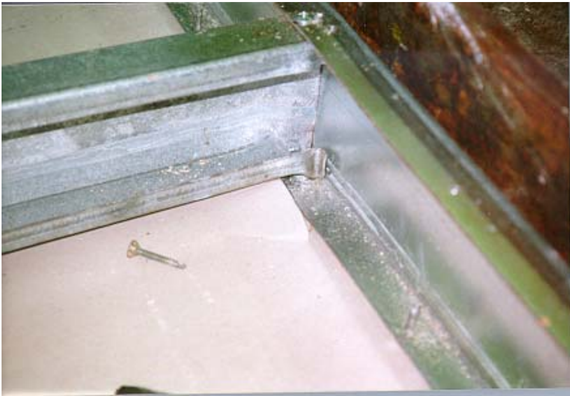
FIGURE 6 Failure of a 2x4x33 mil wall stud by crippling at the end of the stud with 0 psf lateral load (sheathing has been removed).
