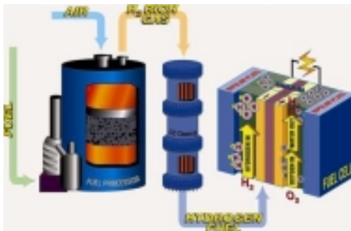
Figure 1: Basic Components of a Fuel Cell
