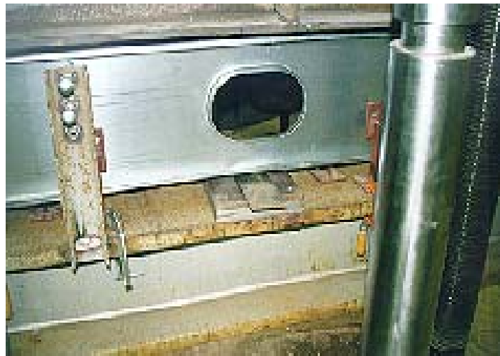
Joist Failure –Combined Shear and bending Test
