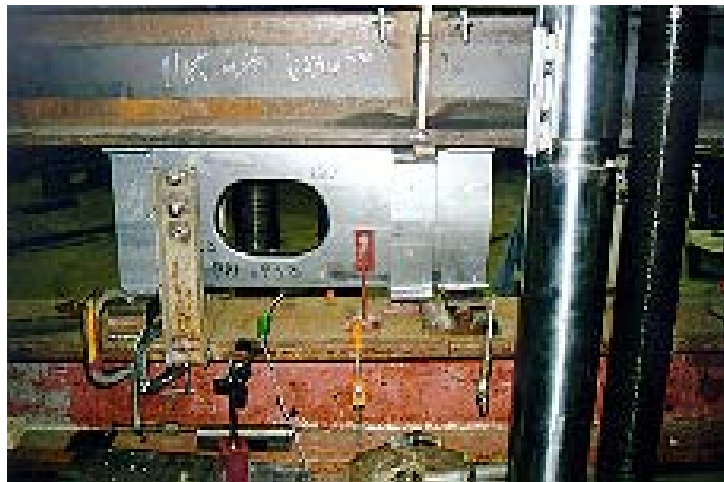
Joist Failure – Shear Test
