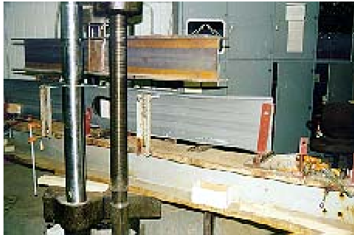
Joist Failure – Combined Shear and Bending
