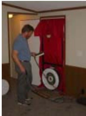
Figure 2-9 Measuring shell leakage with a blower door
