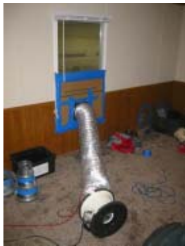
Figure 2-13 Fan simulating clothes dryer exhaust
