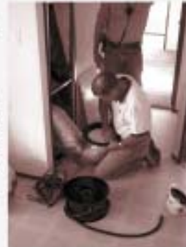
Building scientist installing a calibrated duct fan to measure duct leakage.
