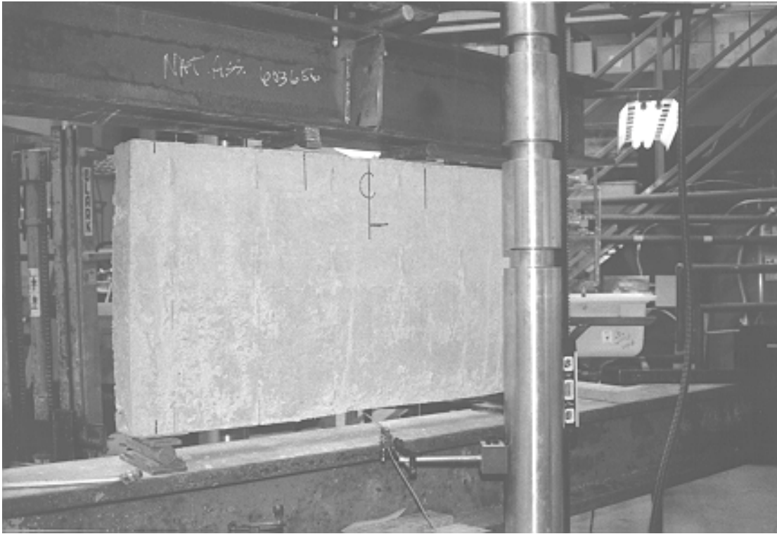
Figure 2 Flat 4x12 Specimen in Universal Test Machine
