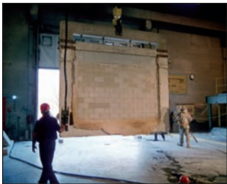
Wood frame and concrete masonry walls after fire test.
