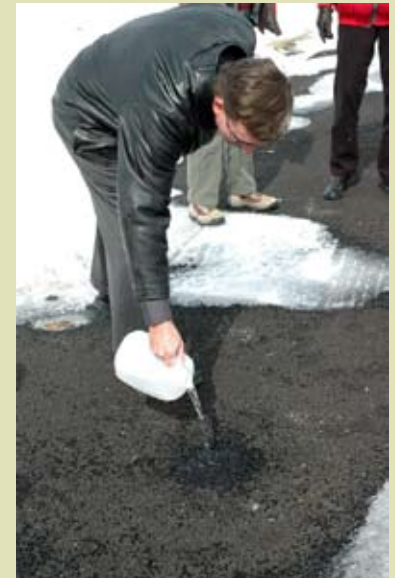
Above left: Difference between permeable asphalt and impermeable asphalt laid side by side for comparison. Above right: Permeable asphalt allows water to seep through.
