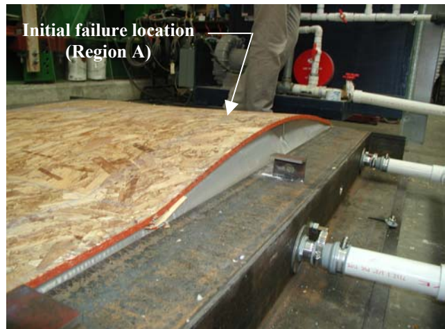
Figure 3.3 – Specimen immediately after failure
