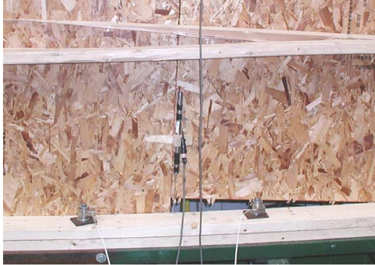
Figure 3.10 – Rafter splitting and tear-through
