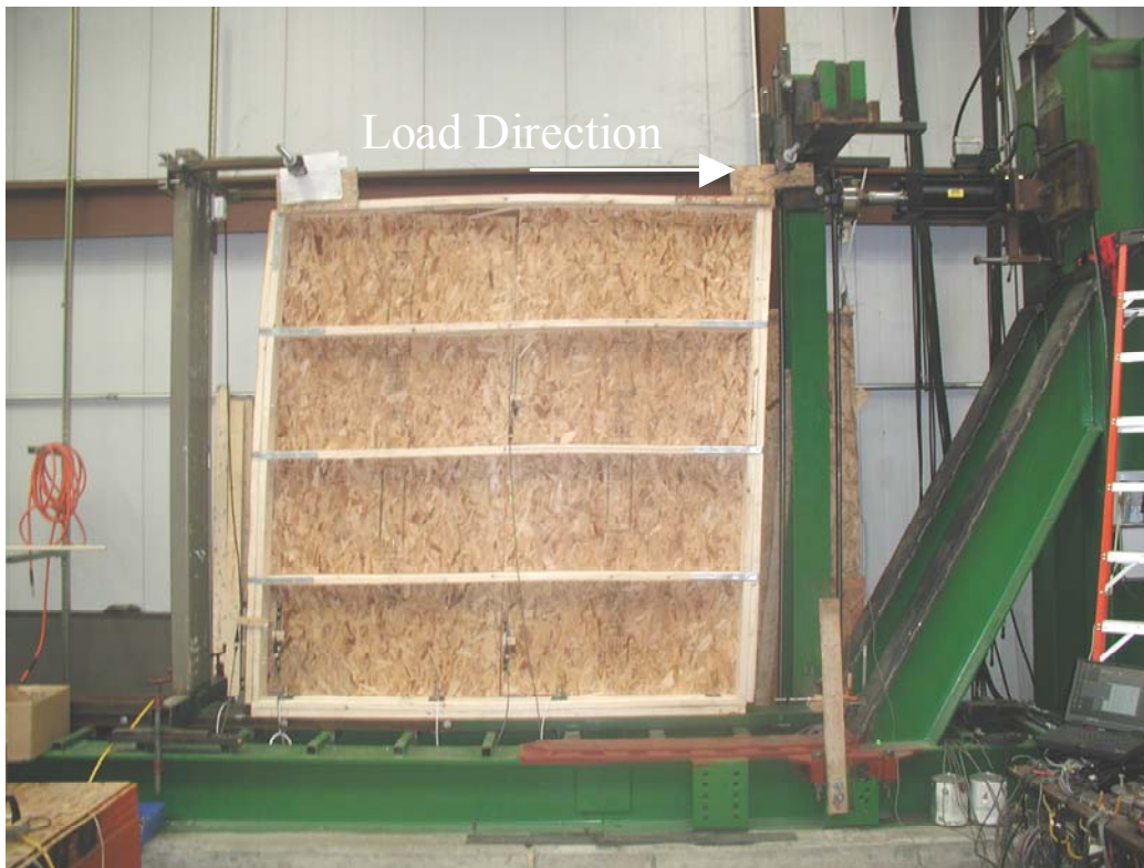
Figure 3.4 – Diaphragm specimen under load
