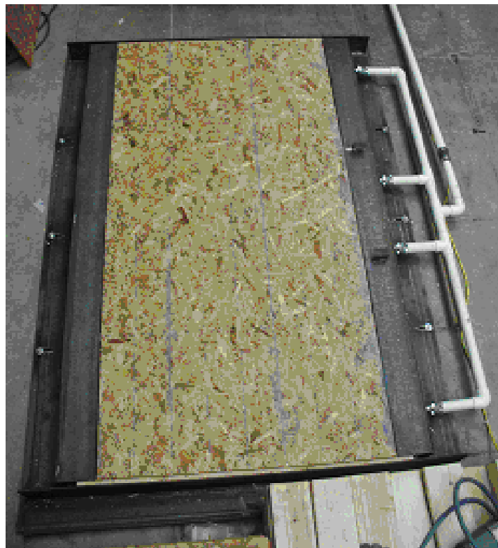
Figure 2.7 – Specimen setup with sheathing attached
