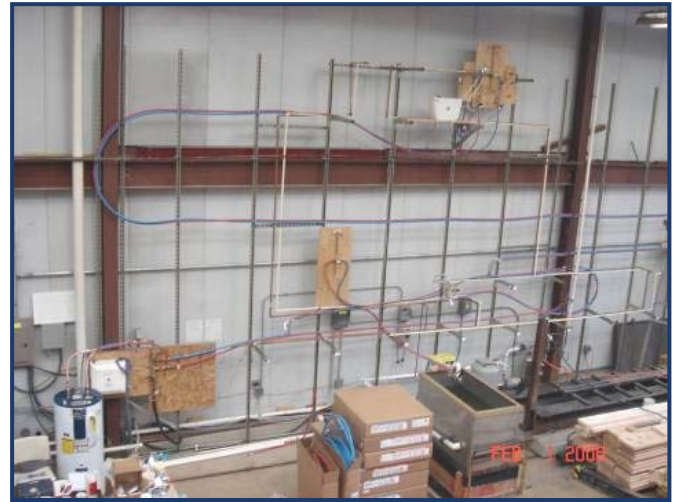
Figure 2 - Laboratory Test Setup for Trunk and Branch System with five fixtures and hot water tank
