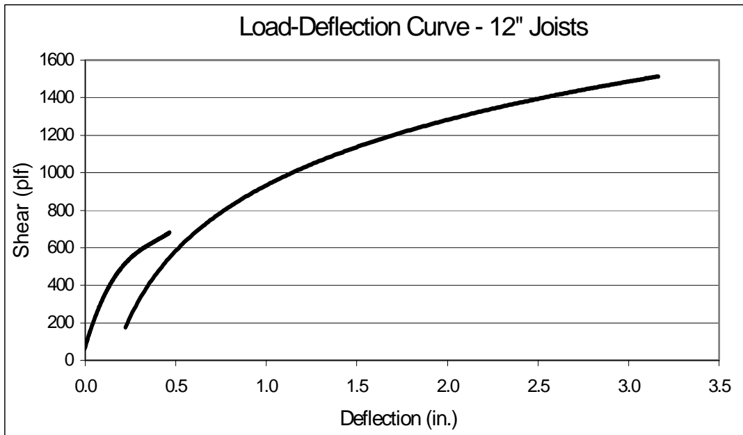
Figure B4 - Shear Load-Deflection Curve for FD12-54-2
