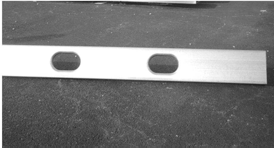
Figure 2 - Web Hole for 8-inch Joist
