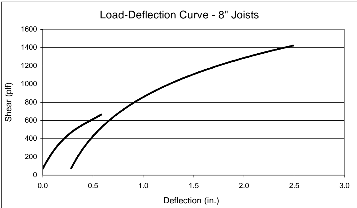
Figure B6 - Shear Load-Deflection Curve for FD8x43-1
