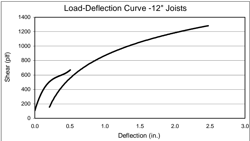
Figure B2 - Shear Load-Deflection Curve for FD12-54-1
