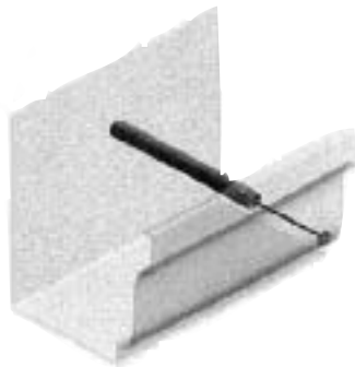
FIGURES 7,8 SPIKE AND FERRULE (FASTENER)
